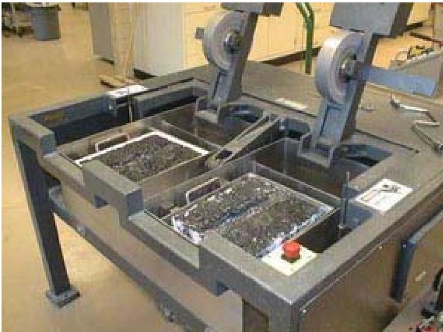
Figure 1. Hamburg Wheel-Tracking Test
