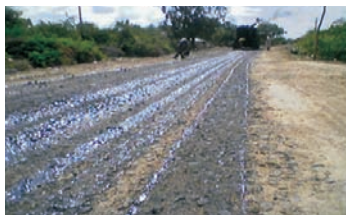
Control - Clogged nozzles. Spluttered spray at 60 – 70 °C
